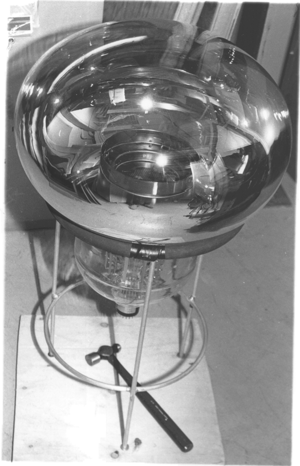
Figure 1.2: The Hamamatsu R1449 20" diameter photomultiplier tube designed for detecting Čerenkov light in water.
